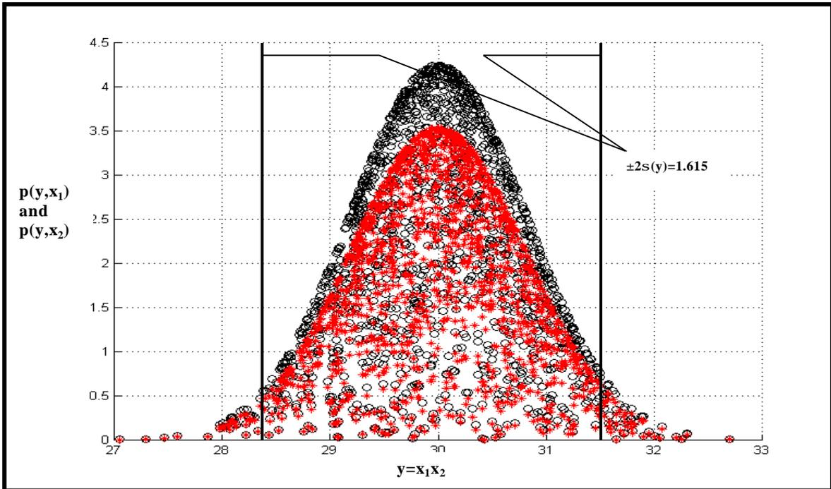
**Figure1 Joint distributions  $p(y, x_i)$  of  $y = x_1x_2$  for uncorrelated inputs  $r_{x_1x_2} = 0$**
