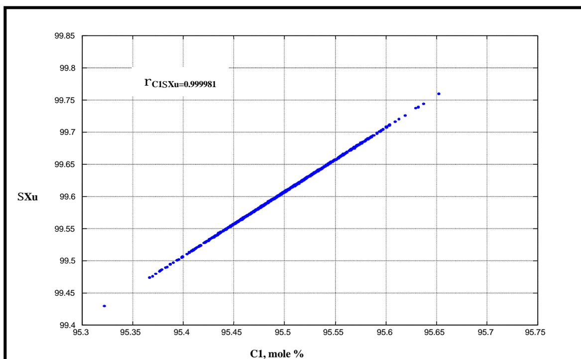
**Figure 5 Un-normalised mole % of C1 versus summation of the un-normalised mole % of all the gas components.**
