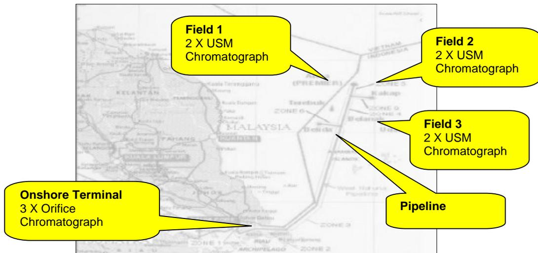
Figure 11 Gas Gathering Pipeline System
