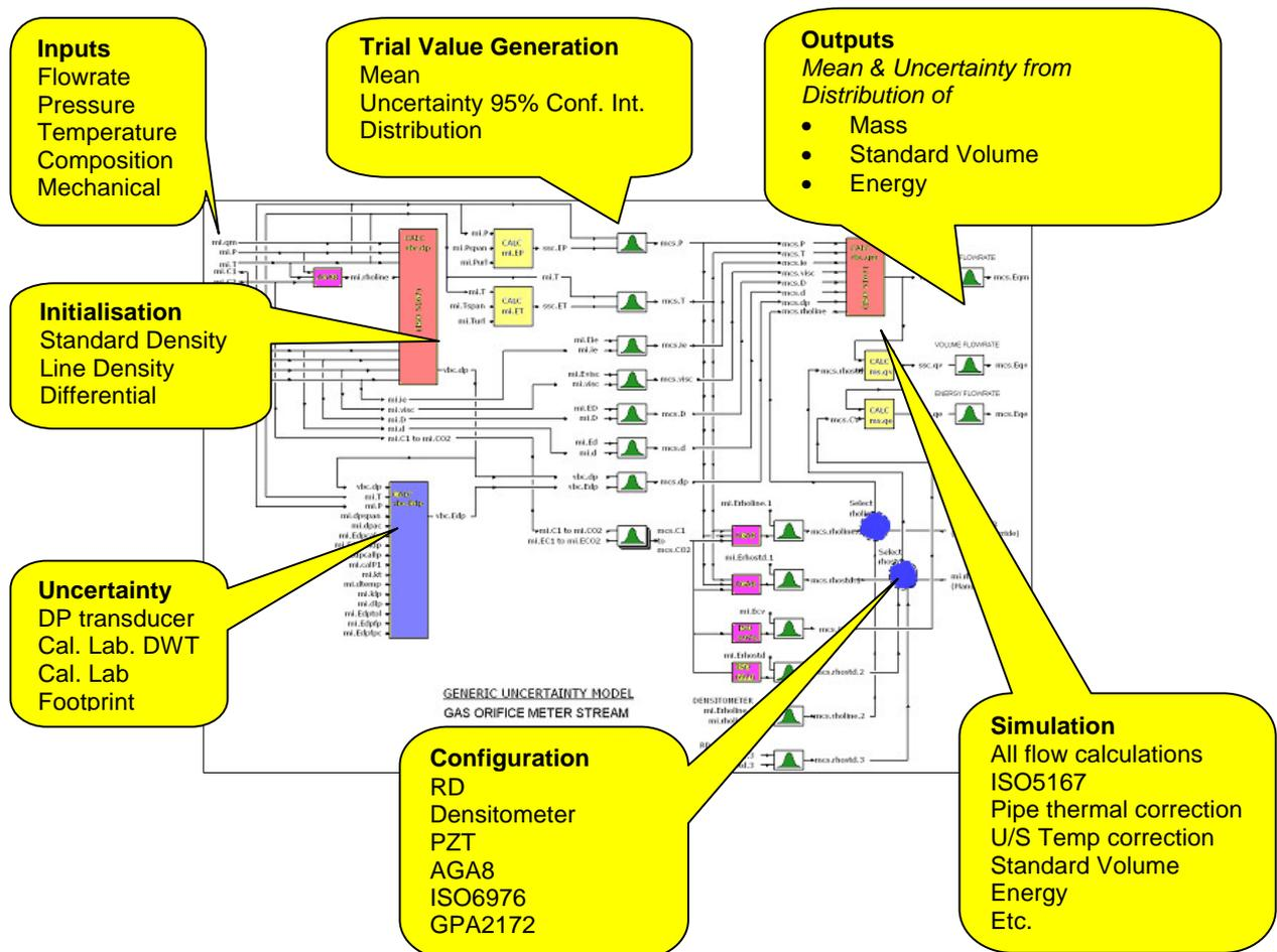
**Figure 6 Fiscal Gas Orifice Plate Meter Generic Uncertainty Model (GUM)**
