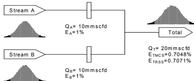
Figure 2 Gas Export Metering System Input Simulation and Model Output Distribution
