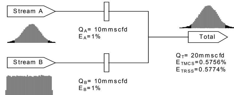
Figure 3 Gas Export Metering System Stream B Rectangular Distribution
